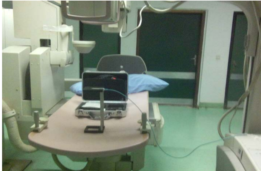
Figure (3) : the x - ray dosimeter at the focus of beam axis of the x - ray table at a focus to image distance of hundred cm , and use minimum field to cover the x - ray dosimeter at the table in radiation department in UROLOGY and NEPHROLOGY center in Mansoura (illustrates the experimental set-up and the instruments used).
